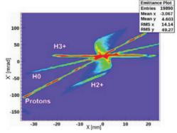
Figure 3: Different particle types separated by solenoid.
