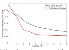
Figure 2: Normalized emittance measured for a proton beam at 45 keV and H beam at 35 keV as a function of the threshold applied to the data.
