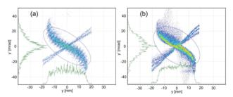
Figure 4: Simulated (b) and measured (a) phase space after the first solenoid, for  $I_{soll}$ =600 A.
