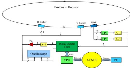
Figure 1: Overview of the Booster transverse digital damper system.
