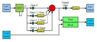
Figure 2: Block diagram of the damping algorithm.
