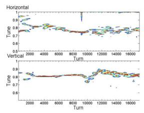
Figure 8: Normalized tune spectrum to enhance small response.
