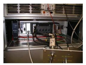
Figure 2: Photo of the opened system. The 8-slot CRIO system is visible as well as the ADC and DIO modules.
