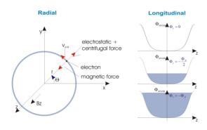
Figure 1: Scheme of the longitudinal and radial confinement principle.
