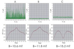
Figure 7: Variation of measured residual gas ion current and light density profile in the region of instabilities (A,C) and in the region of the lens' work function (B),  $\Phi_A$ =4 kV, p=6·10<sup>-4</sup> hPa, He.
