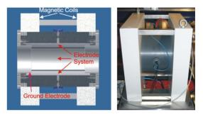
Figure 2: Mechanical drawing (left) and photograph (right) of the space charge lens prototype.
