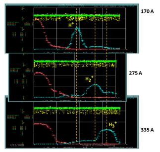
Figure 2: Measurement of ion source species content. Plots show Faraday cup intensities versus spectrometer magnet current. The LEBT downstream solenoid has been optimized to focus individual species to the east Faraday cup. Red curves show west Faraday cup current (straight line) while blue curves show east Faraday cup current (spectrometer line).
