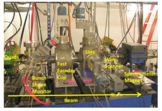
Figure 5: Front-end of the new diagnostics line installed at HINS.
