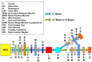
Figure 4: Block diagram of HINS improved diagnostics line for RFQ measurements and future HINS accelerator configurations.
