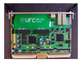
Figure 3: The VME FMC carrier developed at CERN.
