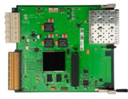
Figure 10: A MTCA .4 FMC carrier developed at DESY
