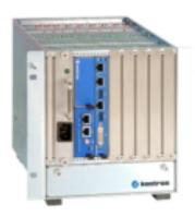
Figure 9: A uTCA crate. In the 1st slot there is the power supply, in the second the MCH and in the 3rd a crate PC.
