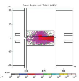
Figure 3: The total power deposited (in mW/g) in the first inter-tank region of the drift tube linac. 15 MeV proton beam hits the beam pipe at 2 degrees incident angle. The beam pipe and the surroundings are estimated to be around 6 cm wide.
