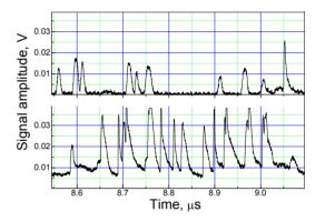
Figure 2: Signal from the single crystal diamond detector. In the upper graph the RF field of the IH was switched on; in the lower graph the IH RF was switched off.
