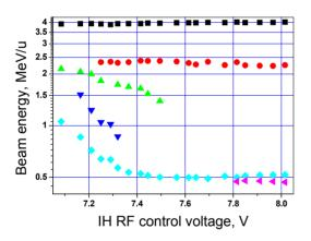
Figure 4: Energy spectra of the ions coming out of IH depending on RF amplitude for a fixed phase of 235°. Black squares shows primary beam, cyan diamonds trends continuously down to the design energy of 0.5 MeV/u. Blue circles, green up-side triangles and blue down-side triangles stand for particles with variable intermediate energy.
