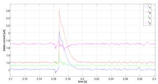
Figure 10: Absolute current reading from each of the blades.
