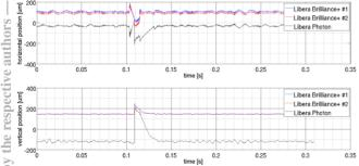
Figure 9: Top-up injection as seen in the photon beam.
