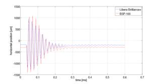
Figure 8: Detailed look at the injection transient during the top-up injection.
