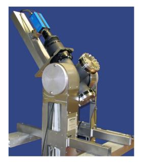
Figure 1: Test stand for optical beam tomography.
