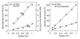
Figure 5: Light output intensity per bunch measured with (a) YAG and OTR screens at 8.4 m downstream of the cathode and (b) YAG and CVD-diamond screens at 19.8 m downstream of the cathode. The beam momentum in these measurements was 24.8 MeV/c.
