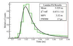
Figure 5: Time distribution of a 0 ps long bunch of electrons once stopped in stainless steel.
