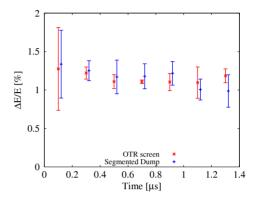
Figure 9: Gated OTR scan measurements, compared with the segmented dump.
