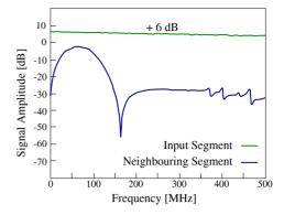
Figure 3: Crosstalk measured with a network analyser.
