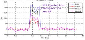
Figure 4: Booster, Transport line BPM sum and DCCT and Storage ring charges during top-up injection.
