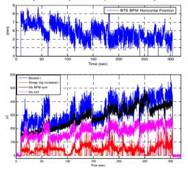
Figure 3: Booster, BTS BPM sum and hor. position and DCCT and Storage ring increased charges.
