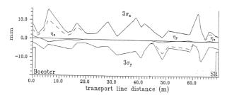
Figure 7: Optical function of Booster to the Storage Ring Transport Line.
