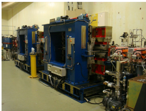
Figure 1: Tandem APPLE-II type undulators installed in the long straight section. Two pink-color magnets at the right side are the kicker magnets.
