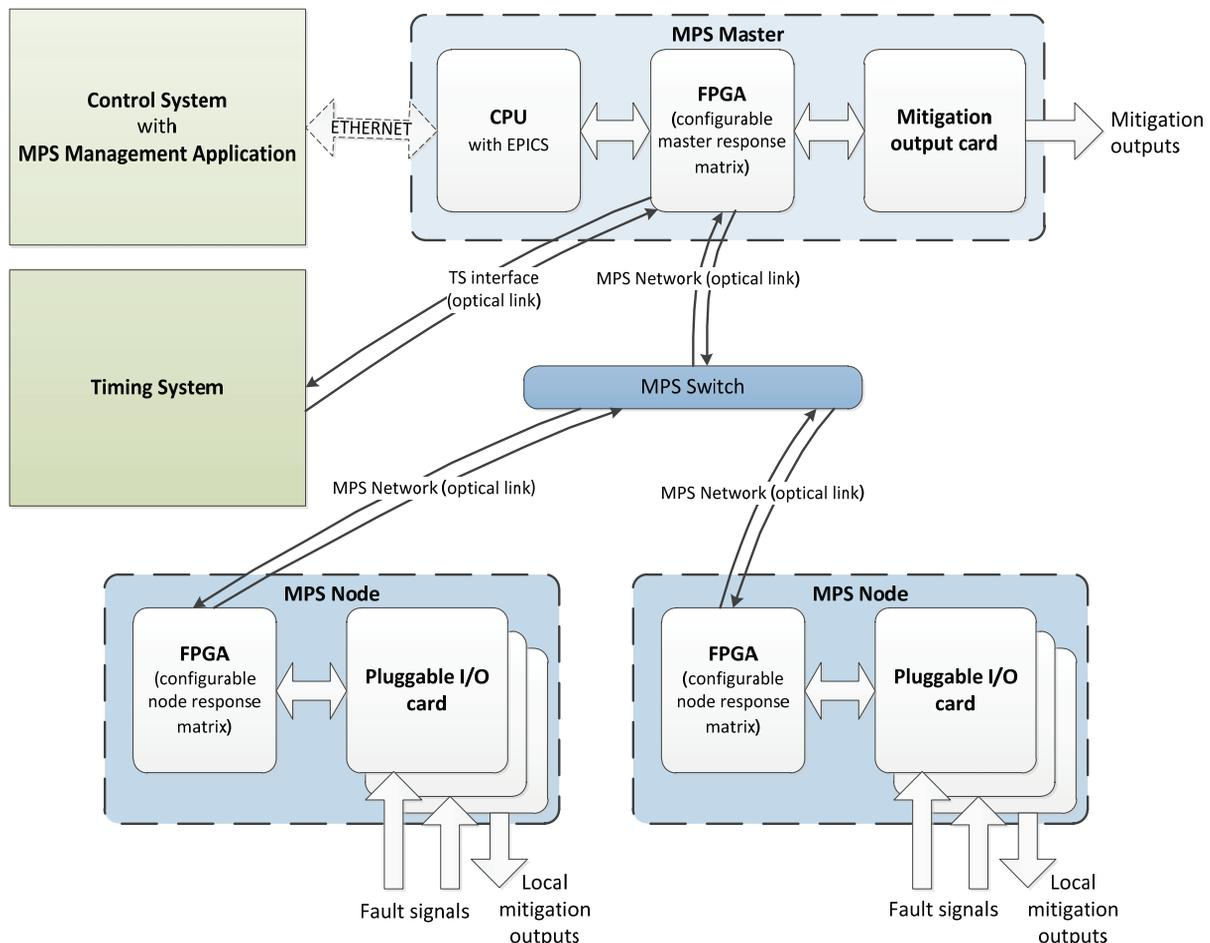
Figure 1: FRIB MPS System Architecture.
