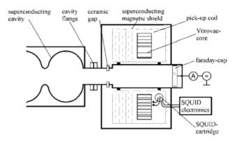
Figure 3: Schematic design of the CCC.
