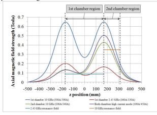
Figure 4: Magnetic field variations of the mirror coils.
