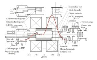
Figure 2: Schematic of the two-chamber Bio-Nano ECRIS with the optimized axial magnetic field distribution.
