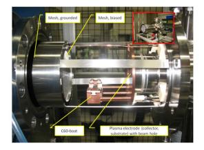
Figure 3: The second (processing) chamber before installation
