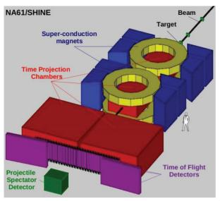
Figure 4: Scheme of the NA61 experiment.
