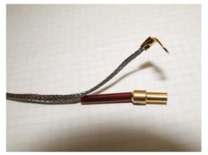
Figure 2: Modified electrical connection for the intermediate electrode.
