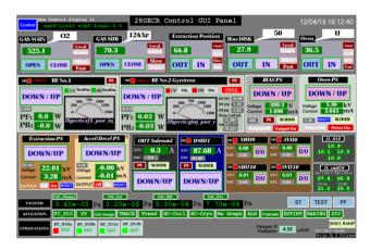
Figure 1: Main control panel constructed with EDM for 28GHz-ECRIS.
