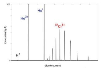
Figure 2: Typical mass/charge spectrum of <sup>54</sup>Cr.
