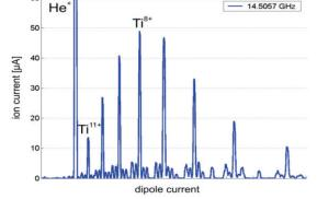
Figure 6: Mass/charge spectrum of natural Ti (forward power = 250 W; reflected power = 28 W; HTO heating power = 234 W).
