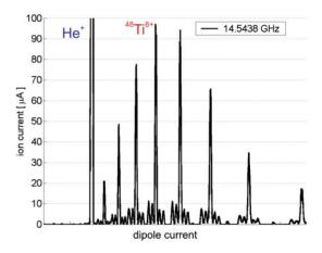
Figure 8: Mass/charge spectrum of natural Ti (forward power = 234 W; reflected power = 95 W; HTO heating power = 262 W).
