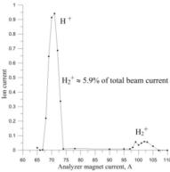
Figure 3: Mass-analyzed ion beam spectrum normalized to the total beam current.
