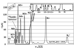
Figure 5: Optimized <sup>40</sup>Ca<sup>16+</sup> (16 µA) spectrum.
