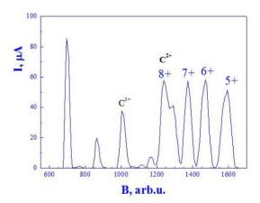
Figure 2: Ti ion spectrum produced by MIVOC method from the DECRIS-4 ion source.
