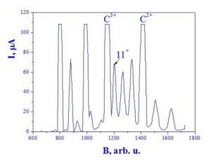
Figure 4: Ti ion spectrum, produced by MIVOC method from the ECR4M source at microwave power of 300 W.
