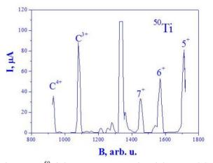
Figure 5: <sup>50</sup>Ti ion spectrum, produced by MIVOC method from the ECR4M source at microwave power of 30 W.
