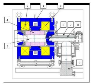
Figure 5: Cross sectional view of the mVinis Ion Source: 1 - the yoke, 2 - the extraction stage coil, 3 - the injection stage coil, 4 - the hexapole magnet, 5 - the plasma chamber, 6 - the additional iron plag, 7 - the injection chamber, 8 - the waveguide, and 9 - the turbomolecular pump.
