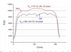
Figure 3: Radial magnetic field distributions for the old and new hexapoles.
