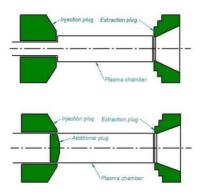
Figure 1: Schematic presentation of the old axial magnetic system (top) and the new axial magnetic system (bottom).
