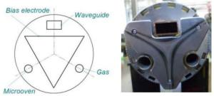
Figure 4: Injection side of the plasma chamber.
