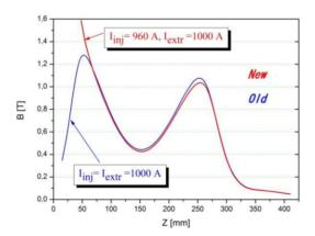
Figure 2: Axial magnetic field distributions for the old and new versions of the magnetic system.
