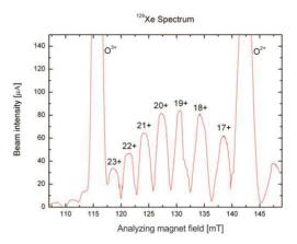
Figure 6: A spectrum of xenon ions optimized for maximal Xe20+ production.
