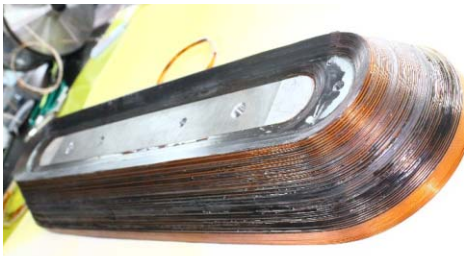
Figure 6: Picture of one of the sextupole coils.
