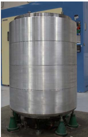
Figure 7: Completed cold mass at the assembly site.
