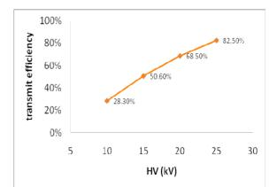
Figure 5: Transmit efficiency of Oxygen beam with different extraction high voltage.
