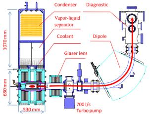
Figure 2:A schematic cross-section view of the LECR4 source body. No mechanical pumping at the injection side for simplicity.
