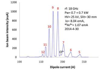
Figure 8: CSD spectrum with the source when optimized on  $Ar^{9+}$  at 1.4 kW.
