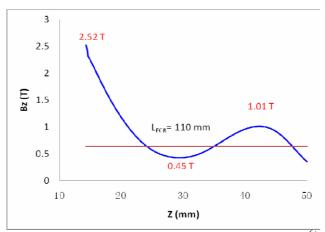
Figure 7: Axial magnetic field distribution when  $O^{6+}$  optimized.
