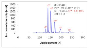
Figure 4: CSD spectrum with the source when optimized on  $O^{6+}$  at 1.0 kW with single rf generator.
