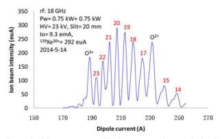
Figure 9: CSD spectrum with the source when optimized on  $Xe^{20+}$  at 1.5 kW.
