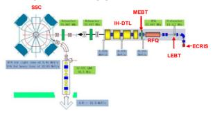
Figure 1: General view of the SSC\_Linac.
