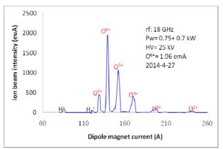
Figure 6: CSD spectrum with the source when optimized on  $O^{6+}$  at 1.45 kW.
