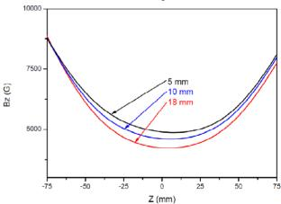
Figure 4: The effect of the soft iron plate thickness.
