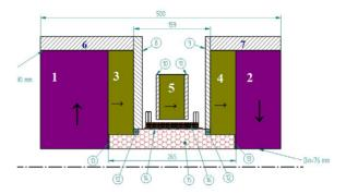
Figure 3: Magnetic structure of DERIS-PM. 1÷5 – PM rings; 6, 7 – soft iron rings; 8÷11 – soft iron plates, 12÷14, 16 - auxiliary elements, 15 – hexapole.
