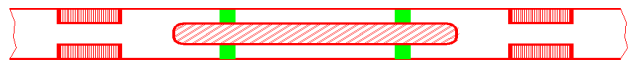
Figure 6. A cross-sectional side-view of the one-third structure used for tests. Green lines represent matching slabs. FE rods are not seen in this cross-section.
