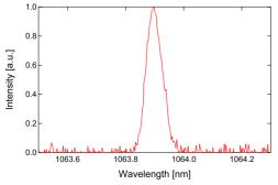
Figure 11: Optical spectrum of 1.2GHz pulse.
