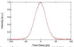
Figure 12: Autocorrelation trace of 1.2GHz pulse.
