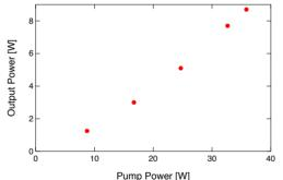
Figure 10: Input and output characteristics of the 1.2GHz laser system.
