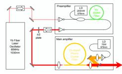
Figure 2: Schematic of Yb fiber laser amplifier system.
