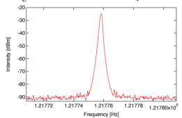
Figure 9: RF spectrum of Nd:YVO<sub>4</sub> oscillator pulse.
