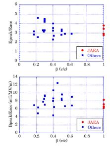
Figure 5: Epeak/Eacc (upper) and Bpeak/Eacc (lower) as a function of  $\beta$ . Solid circles: our spoke cavity design and solid squares: other spoke cavities shown in references [4-5].
