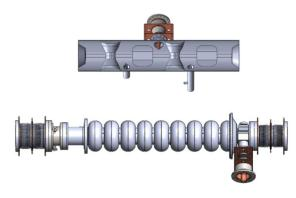
Figure 1: Schematic views of spoke cavity (upper) and elliptical cavity (lower).
