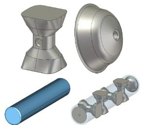
Figure 2: Example of parts of spoke cavity; spoke (upper left), tank (lower left) and end nose (upper right) and their assembly (lower right).
