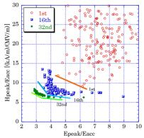
Figure 3: Distribution (dots) and Pareto fronts (lines) of Epeak/Eacc and Hpeak/Eacc at some generations.
