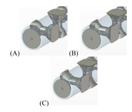
Figure 4: Typical shapes of spoke cavity near Pareto front of Epeak/Eacc-dominant (A), Hpeak/Eacc-dominant (C) and their medium (B).
