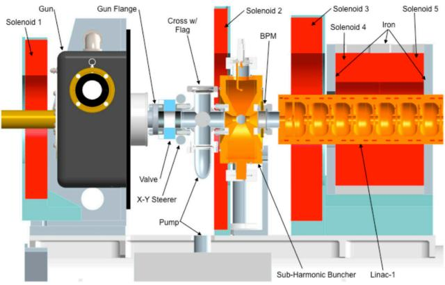
Figure 3: FHI FEL front-end configuration.
