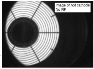
Figure 10: Gun filament and grid.
