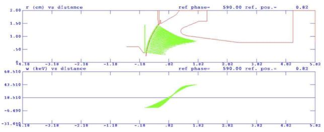
Figure 5: TStep radial projection (upper) and energy profile (lower) during bunch formation from the gun.
