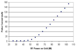
Figure 8: Pulse current with RF power on the grid.
