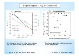
Figure 9: To increase the coercivity in the grain, the best way is to decrease the magnet temperature. (a) The coercivity increases with the temperature decrease. (b) Resistance against the radiation remarkably increases at low temperature.
