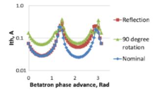
Figure 4: BBU threshold currents for different amount of betatron phase advance and coupled motion of x and y planes in tranverse phase space using reflectors (skew quadrupoles) or solenoids [8].
