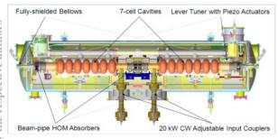
Figure 1: CW-ERL cryomodule under development.
