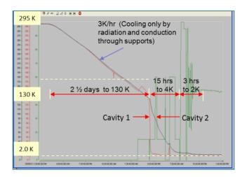
Figure 5: Cool-down to 2K. The red and black curves indicate the temperatures of the two cavities and the green curve shows position of the liquid helium feed valve.
