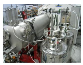
Figure 2: Fully assembled cryomodule undergoing Oualification tests.
