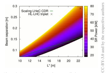
Figure 9: Expected total synchrotron radiation power as a function o the location of the first focusing element for the lepton beam next to the experiment  $(L^*)$ .
