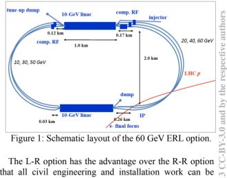
Figure 1: Schematic layout of the 60 GeV ERL option.
