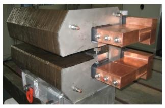
Figure 4: CERN prototype for a normal conducting LHeC dipole magnet.
