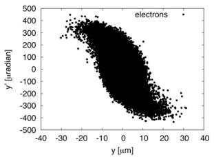
Figure 11: Simulation studies for the damping of transverse beam oscillations in the presence of cavity Wakefields and a linearized beam-beam force at the interaction point.
