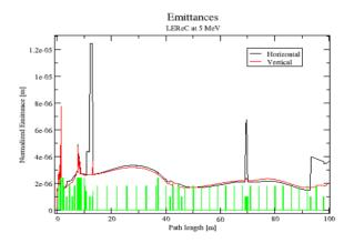
Figure 8: Normalized rms emittances. The spike in the horizontal emittance at the path length of 12 m is caused by the dispersion of the zig-zag merger.
