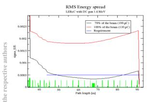
Figure 6: Energy spread in the cooling sections. The requirement is fulfilled.
