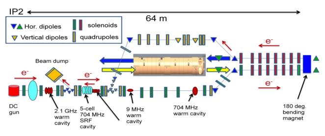
Figure 2: Layout for Phase II.
