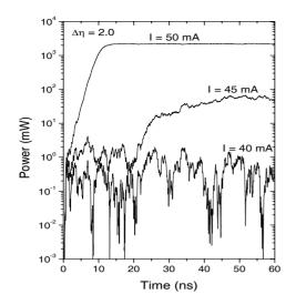
Figure 3: Evolution of power in the surface mode in SP-BWO for different values of beam current as calculated by numerical simulation. Parameters used in the numerical simulation are described in the text.
