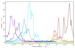
Figure 2: Measured spectra when tuning the wavelength by varying the undulator gap over the spectral gap around  $29 \mu m$ .
