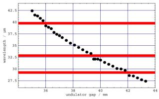
Figure 3: Wavelength versus undulator gap measured at 40 MeV electron beam energy. Even though the lasers is working for almost all settings of the undulator gap, some wavelengths are inaccessible (like 29  $\mu$ m or 33  $\mu$ m) which are shown with red stripes.
