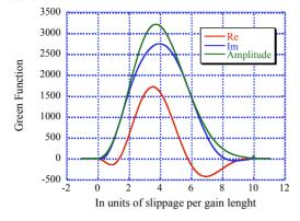
Figure 3: The amplitude, the real and the imaginary part of the Green function envelope after propagation in FEL with ten-gain length. For comparison with 3D FEL in the following section – their one gain length is equal and 2 m or 40 periods for amplitude. Thus, the unit slippage in this figure corresponds to 40 optical wavelengths.
