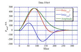
Figure 7: The Green-function envelope calculated by RON at z=20m, i.e. after 10 gain-length FEL, resembles all the features seen in the 1D case (Fig.3).
