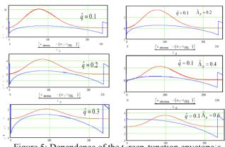
Figure 5: Dependence of the Green-tunction envelope's amplitude (red line) and its phase (blue line) on energy spread  $\hat{q}$  parameter and on space charge  $\hat{\Lambda}_p$  parameter (see definitions in [8]). Horizontal axis is in units of optical wavelengths. Total slippage is 240 wavelengths.
