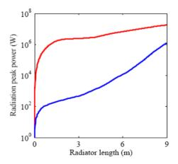
Figure 4: The peak power growth in superradiant harmonic operation of SDUV FEL. Red is the 3<sup>rd</sup> harmonic 87.3nm and blue is the fundamental 262nm.
