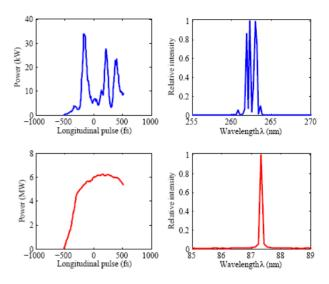
Figure 3: The output FEL performance after 4 segments radiator in linear harmonic operation of SDUV FEL.
