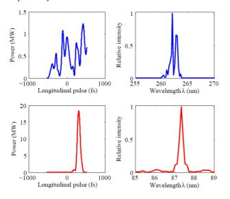
Figure 5: The final output performance in superradiant harmonic operation of SDUV FEL.
