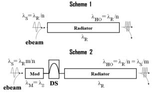
Figure 1: Layout of harmonic operation.
