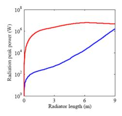
Figure 2: The peak power growth in linear harmonic operation of SDUV FEL. Red is the 3<sup>rd</sup> harmonic 87.3nm, and blue is the fundamental 262nm.
