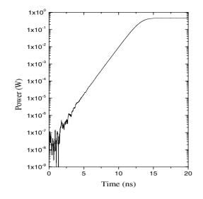
Figure 3: Evolution of power in SP-BWO for the parameters mention in the text. The electron beam current is assumed to be 12 mA.
