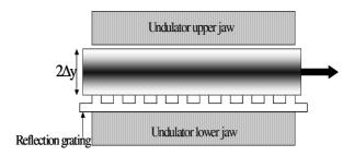
Figure 2: Schematic of focusing in a Smith-Purcell BWO using Undulator.
