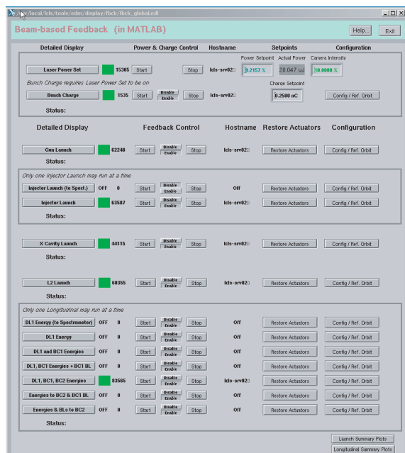
Figure 2: Beam-based Matlab-EPICS feedback front page.
