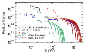
Figure 6: Peak Brilliance of ARC-EN-CIEL (10 kHz assumed for phase 2, 20 mA average current for phase 3).
