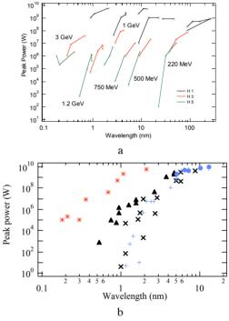
Fig. 5: Spectral range covered by the HHG seeded FEL sources of ARC-EN-CIEL a) Wide spectral range : fundamental (black), third (red) and fifth (green) harmonics of the radiator b) Short wavelength spectral range : Seed 30-50 kW, 50 fs-FWHM: LEL1 (Phase 2), (+) planar (o) helical configuration ; LEL2 (x) E=1 GeV, ( $\Delta$ ) E=1.2 GeV; \* LEL4 in Phase 3.
