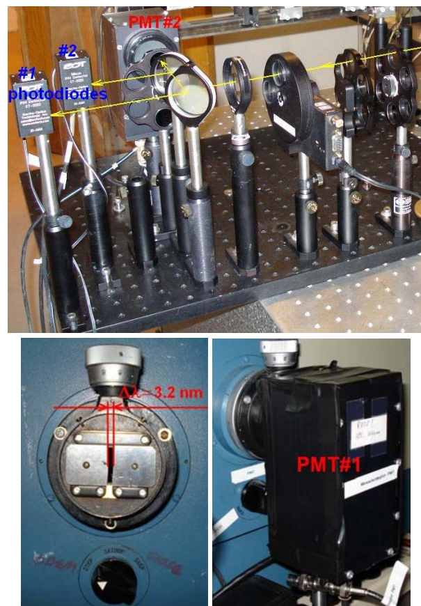
Figure 3: (Upper photo): a four-stage FEL gain measurement bench with two photodiodes and two PMTs. (Lower photos): the 1 st stage PMT receives the optical beam after a monochromator with its exit slit opened to about 3.2 nm.
