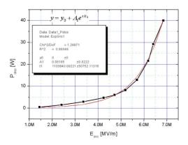
Figure 5: RF power dissipation vs. gradient.
