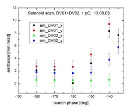
Figure 15: Normalized transverse emittance as function of laser phase for 1 pC bunch charge.
