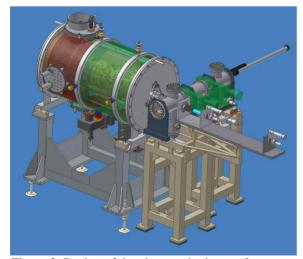
Figure 3: Design of the photo cathode transfer system.
