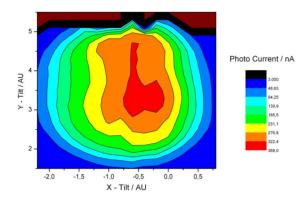
Figure 9: Q.E. map of the Cs<sub>2</sub>Te photo cathode in the SRF gun. Photo current measured in the Faraday cup.
