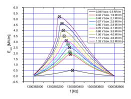
Figure 7: Measurement of the cavity resonance curve (gradient vs. frequency) for increasing input power.
