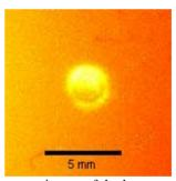
Figure 8: CCD camera image of the laser spot at the virtual cathode. The spot diameter is 2.7 mm.
