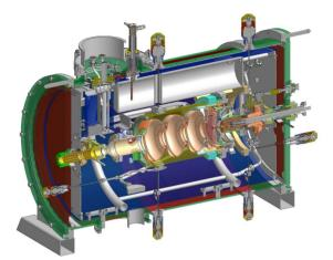
Figure 1: Design of the SRF Gun cryomodule.
