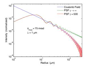
Figure 2: Point spread function of the OTR source distribution for a lens acceptance angle of 75 mrad. Shown are the Coulomb field for  $\gamma=500$  and the PSF at the same  $\gamma$  and for  $\gamma\to\infty$ .
