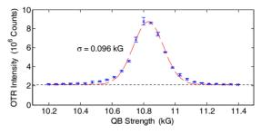
Figure 3: OTR intensity (lower) and beam sizes (upper part) measured downstream of BC1 at OTR12 as a function of the dispersion correction quadrupole (QB) in the first dogleg with no bunch compression. The vertical line indicates the peak of the OTR intensity curve.
