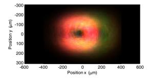
Figure 9: Comparison of observed and simulated COTR color images.
