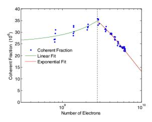
Figure 5: Fraction of the bunch charge radiating coherently as a function of charge. A linear and an exponential fit are used below and above  $2.8 \times 10^9$  electrons.
