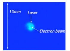
Figure 3: Transverse overlap between the 800 nm laser and the electron beam observed on the OTR screen.
