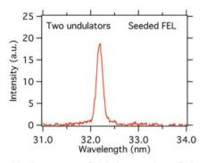
Figure 11: Spectrum of 5th harmonics of the seeded FEL, the electron bunch length is 4 ps.
