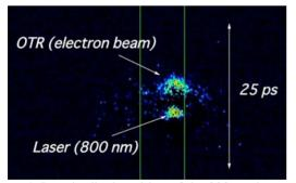
Figure 4: Longitudinal position of the 800 nm laser and the electron bunch measured with a streak camera. Two pulses are intentionally displaced in the figure.
