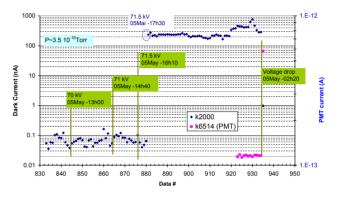
Figure 2: Dark current (label K2000) and PMT level (label K6514) of SS electrodes at 1 mm gap.
