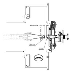
Figure 3: Diode Configuration inside the 500 kV pulser UHV chamber. The cathode is mounted on the left side.
