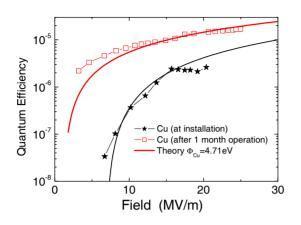
Figure 5: QE increase for a Cu cathode after 1 month of laser and high voltage operation.
