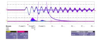
Figure 4: Measured waveform of the HV pulse 280 kV (upper trace) and X-ray scintillator signal lower trace.
