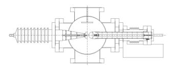
Figure 1: Diode configuration of the 100 kV DC chamber. The cathode is flat the anode is hemispheric and the third flat electrode above is used for plasma glow discharge.
