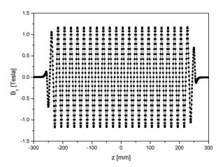
Figure 2: The calculated field profile.
