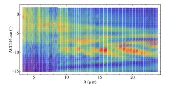
Figure 3: Normalized spectral intensity for  $3 \mu m < \lambda < 24 \mu m$  as function of the off-crest phase of the first acceleration module. Each wavelength bin is normalized to its maximum value individually. A typical FEL operation point is at  $-4^{\circ}$  to  $-6^{\circ}$  off-crest.
