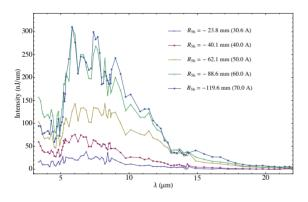
Figure 10: Intensity of coherent transition radiation in oncrest mode of both bunch compressors. The first magnetic chicane is set to nominal operation conditions while the dipol strength of the second chicane is varied.
