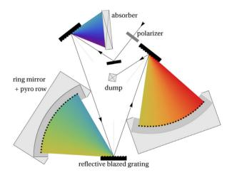
Figure 1: Schematic layout of the two stage single shot spectrometer.
