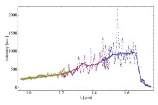
Figure 7: Single shot (dots) and averaged (line) CTR spectrum between 0.95  $\mu$ m and 1.7  $\mu$ m measured with a commercial InGaAs spectrograph. The response of the detector is basically flat between 1.0  $\mu$ m and 1.7  $\mu$ m.
