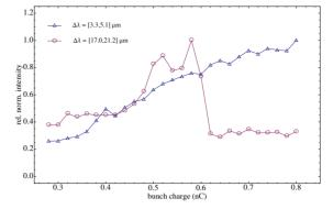
Figure 4: Normalized spectral intensity for two wavelength bands as function of the bunch charge. The band  $3.3 - 5.1 \,\mu\text{m}$  is dominated by microstructures while the band  $17 - 21 \,\mu\text{m}$  results predominantely from the leading current spike of the compressed bunches.
